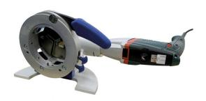
All multifunctional tools (MFW) are two-sided tool bits with protective coating against tool wear. This enables the preparation of tubes made of high-alloy, unalloyed and low-alloy steels and aluminum with high precision very quickly and efficiently.
